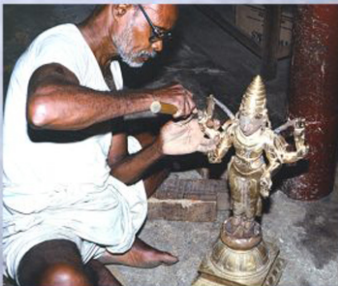
Sthapati or icon maker from Swamimalai, Tamil Nadu finishing an image made by the lost wax process
